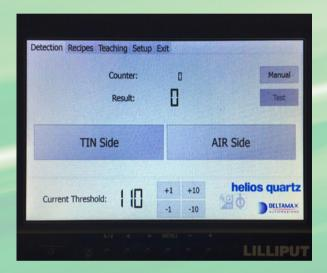
production line's control panel, instantly signaling with a green LED if it is scanning the air side; while, if the device scans the "tin side", a red LED flashes. The device has an open contact and the customer can connect it to the control panel of the line and decide to translate this signal into an alarm sound or even a direct command to block the line, thus allowing the operator to place the glass sheet in the right position.
