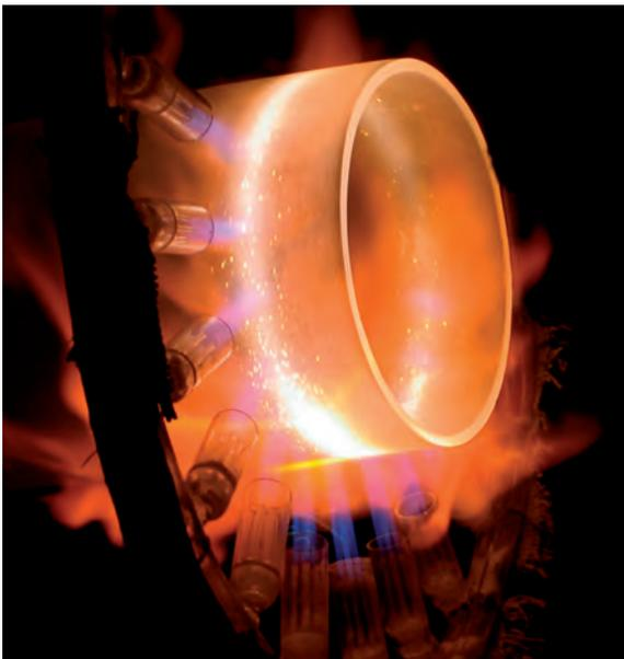
H<sub>2</sub>/O<sub>2</sub> flame fusion production method
