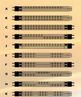
Helios Quartz Technical Department can realize twin tube IR emitters with different filament configuration. This allows extraordinary flexibility both in terms of heated area modularity and lead wire position. In the picture aside there are represented some of the most common filament configuration.
