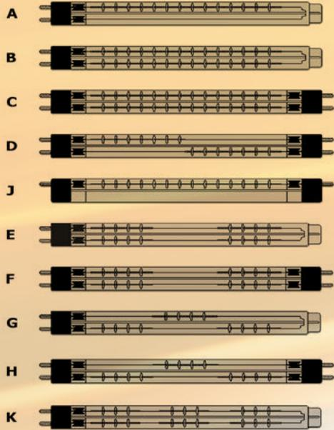
Helios Quartz Technical Department can realize twin tube IR emitters with different filament configuration. This allows extraordinary flexibility both in terms of heated area modularity and lead wire position. In the picture aside there are represented some of the most common filament configuration.
