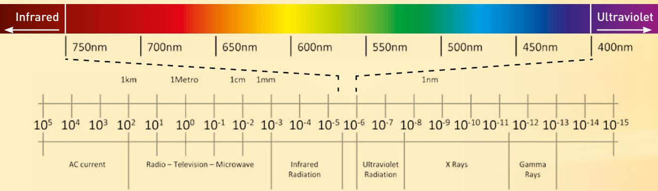
In particular, the infrared wavelengths range generated by the IR quartz emitters, are located in the range of 3,5  $\mu\text{m}$  (medium wave) and 0,9  $\mu\text{m}$  (short wave). Depending on the type of material to be heated it is possible to use different types of IR wavelengths to reach the maximum propagation of energy and to obtain a faster and more efficient heating process.
