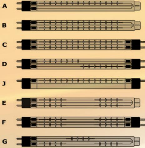
Helios Quartz Technical Department can realize twin tube IR emitters with different filament configuration. This allows an extraordinary flexibility both in term of heated area modularity and cables position. In the picture aside there are represented some of the most common filament configuration.
