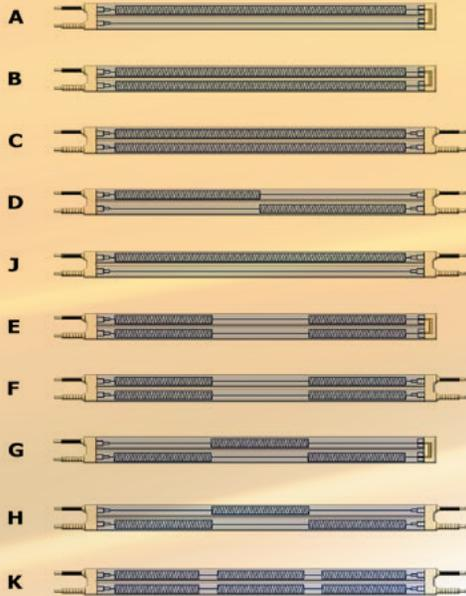
Helios Quartz Technical Department can realize twin tube IR emitters with different filament configuration. This allows an extraordinary flexibility both in term of heated area modularity and cables position. In the picture aside there are represented some of the most common filament configuration.
